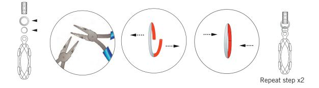
STEP 2: Open two 6mm jump rings with flat nose pliers. Attach one 6mm jump ring to a 4mm jump ring, the SWAROVSKI ELEMENTS Pendant, art. 6015/A and the 2nd 6mm jump ring.
